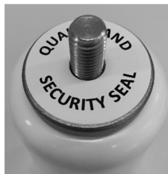
Factory made, intact
